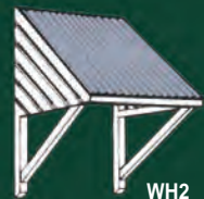
WH2 Diagonal Skillion overhang 565mm Height 1300mm
